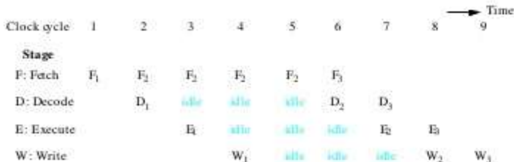
(b) Function performed by each processor stage in successive clock cycles
