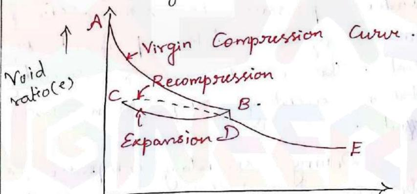
At any intermediate stage at B, the pressure is completely removed, the sample expands as represented by the expansion curve BC.
