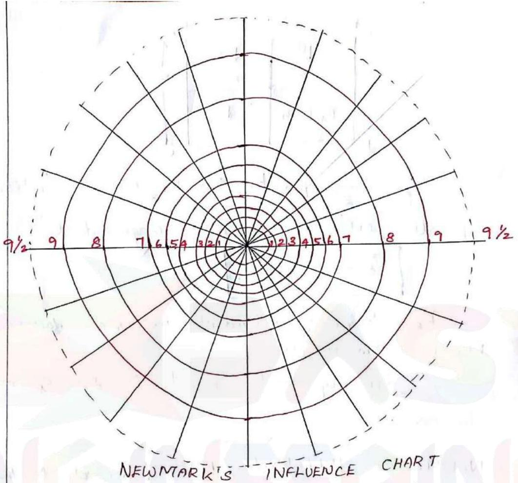
Let a uniformly loaded circular area of radius  $r_1$ , cm be divided into 20 sectors (area units). If  $\sigma_r$  is the intensity of loading and  $\sigma_z$  is vertical pressure at depth  $z$  below centre of area, each unit such as OA, OB, etc., exerts a pressure equal to  $\sigma_r/20$  at centre.
