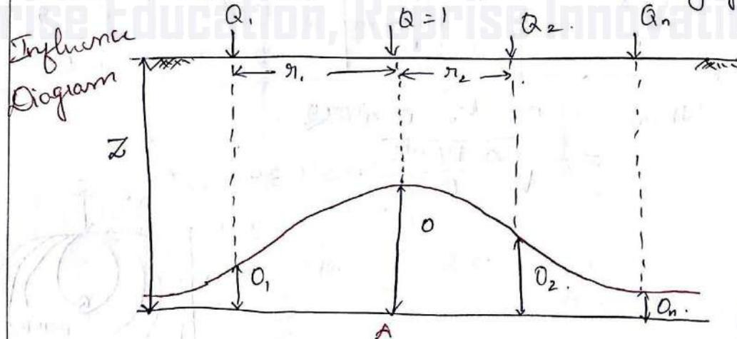
Such a diagram is helpful in (Q) computing the vertical stress  $\sigma_z$  at A due to number of concentrated loads  $Q_1, Q_2, \dots, Q_n$  situated at radial distances  $r_1, r_2, \dots, r_n$  from vertical axis through point A.
