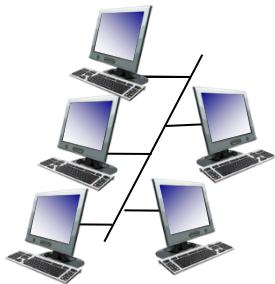
shared wire (e.g., cabled Ethernet)
