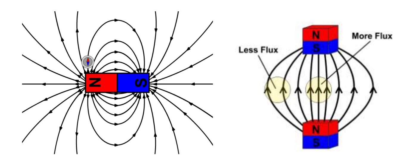
Magnetic Flux is a measure of the number of magnetic field lines passing through a given point.
