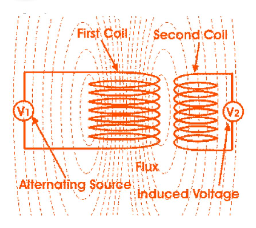
Mutual Inductance is the property of two coils, by virtue of which, either of the two coils opposes any change in the strength of the current flowing through the other coil, by inducing an opposing emf in itself.
