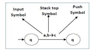
This means at state q<sub>1</sub>, if we encounter an input string 'a' and top symbol of the stack is 'b', then we pop 'b', push 'c' on top of the stack and move to state q<sub>2</sub>.
