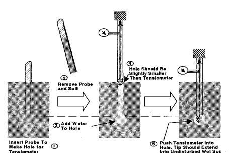
undisturbed soil just below the depth created by the probe. After the probe has been installed, the soil and porous tip usually reach equilibrium within 24 hours, and the instrument is then ready to use.
