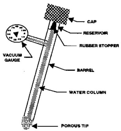
cohesive forces between adjacent water molecules. As the suction approaches approximately 0.8 bar (80 cb), the cohesive forces are exceeded by the suction and the water molecules separate. When this occurs, air can enter the tube through the porus tip and the tensiometer no longer functions correctly. This condition is referred to as breaking tension. Tensiometers work in the range from 0 to 0.8 bar. The suction scale
