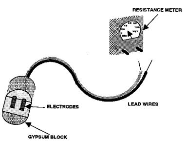
electrical resistance) indicate high levels of soil-water, whereas low meter readings indicate low levels.
