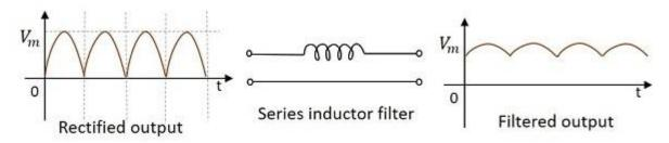
The rectified output when passed through this filter, the inductor blocks the ac components that are present in the signal, in order to provide a pure dc. This is a simple primary filter.
