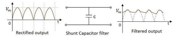
The rectified output when passed through this filter, the ac components present in the signal are grounded through the capacitor which allows ac components. The remaining dc components present in the signal are collected at the output.
