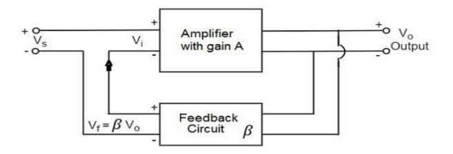
From the above figure, the gain of the amplifier is represented as A. the gain of the amplifier is the ratio of output voltage  $V_o$  to the input voltage  $V_i$ . The feedback network extracts a voltage  $V_f = \beta V_o$  from the output  $V_o$  of the amplifier.
