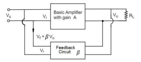
As the feedback circuit is connected in shunt with the output and the input as well, both the output impedance and the input impedance are decreased.
