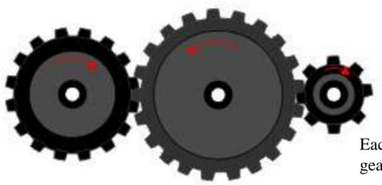
Each shaft carries only one gear wheel.
