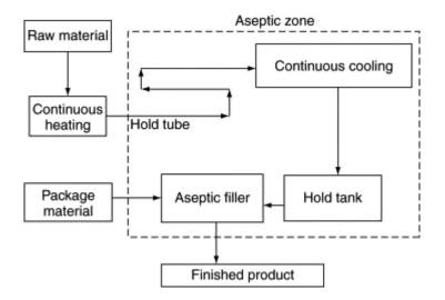
Aseptic packaging systems fill sterile product into sterile packages within the confines of the sterile zone of the filler. The aseptic zone/sterile zone extends from the point where sterilized packaging enters the sterile zone to where the sealed package is evacuated. Common attributes to all aseptic packaging systems include:
