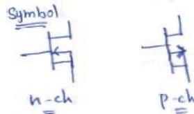
\* MOSFET is also referred to as an IGATE because the gate is isolated from the channel.
