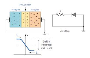
The potential barrier that now exists discourages the diffusion of any more majority carriers across the junction. However, the potential barrier helps minority carriers (few free electrons in the P-region and few holes in the N-region) to drift across the junction.
