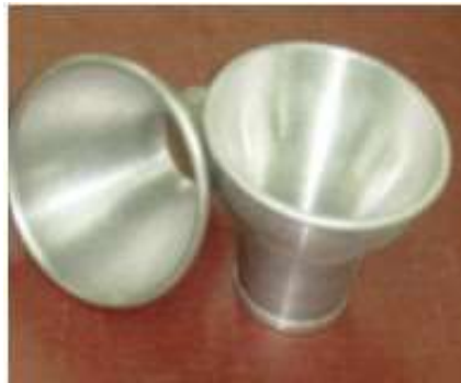
Fig. 412: Manual funnels for stuffing of larger calibre sausages, made of food-grade aluminium
