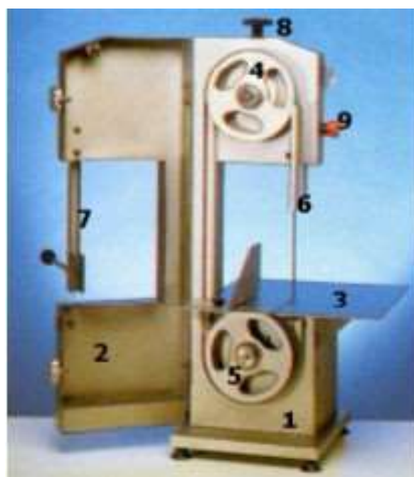
Fig. 404: Band saw open 4 – adjustable tensioning wheel 5 – drive wheel (connected to motor) 6 – band saw blade guide 8 – tensioning knob 9 – emergency switch
