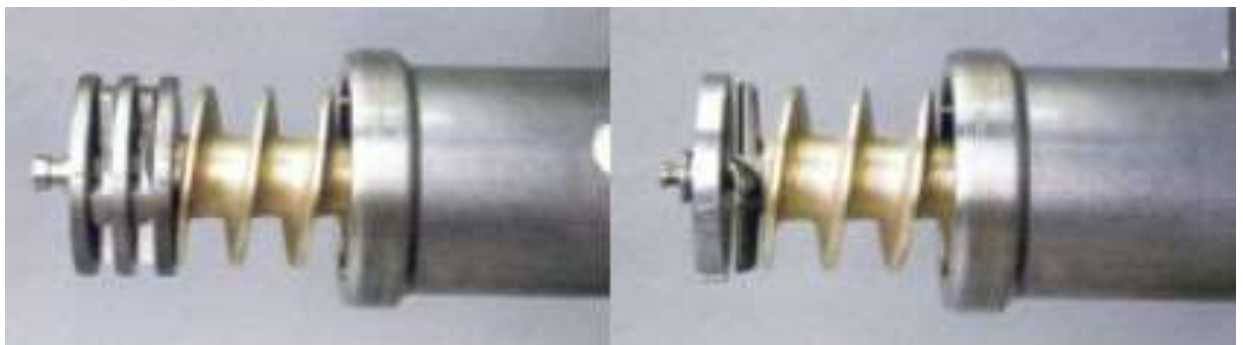
Fig. 393: Cutting sets in meat grinders, assembled on feeding worm (auger) Left: UNGER five-piece cutting set Right: ENTERPRISE two-piece cutting set
