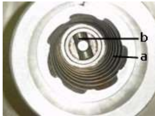
Fig. 394: Feeding auger housing: Critical areas for cleaning are the throat (a) in the housing and the connection point of feeding worm and drive shaft
