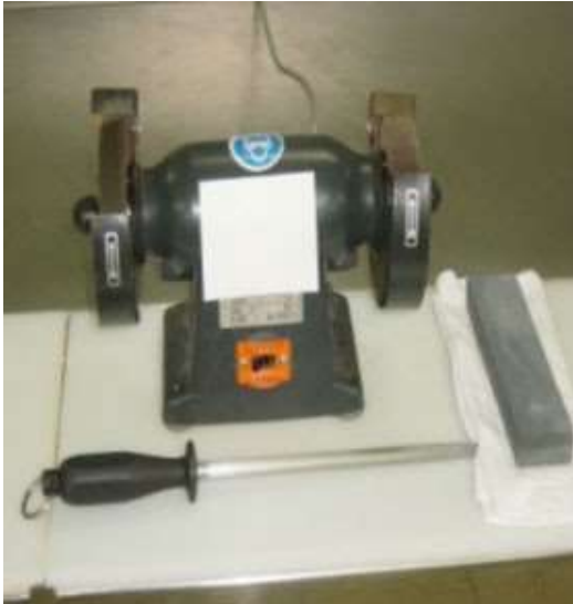
Fig. 389: Knife sharpening machine with sand-paper flap-wheel for grinding (right) and whetting (left) Right side: wet stone for sharpening Below in front: polishing steel
