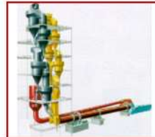
Preheater and Kiln
