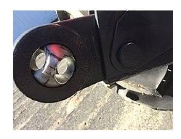
Adjustable three-point ball on lift arm. Ball may be rotated to fit either Category I or II implements
