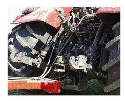
Rear three-point hitch of a Case IH tractor with implement attached by the drawbar
