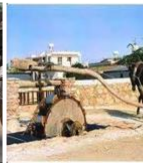
Persian wheel- water lifting
