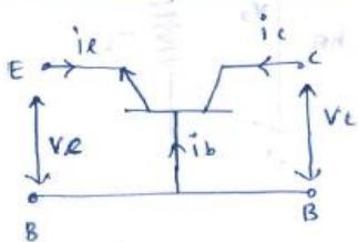
$$(1) \Rightarrow V_c = h_{1e} i_e + h_{rb} V_b \quad \text{--- (5)}$$
