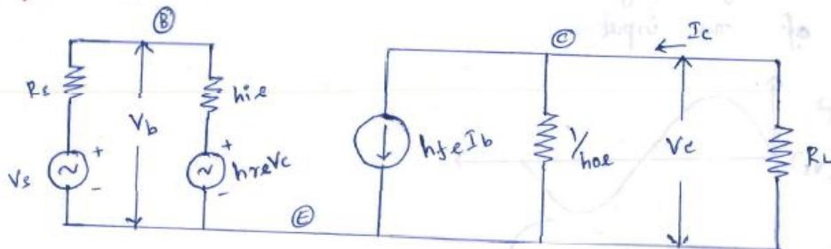
Here,  $\frac{1}{h_{re}} \parallel R_L$  & if  $\frac{1}{h_{re}} \gg R_L$ , then  $h_{re}$  may be neglected.
