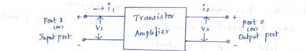
\* From 4 variables  $v_1, v_2$  &  $i_1, i_2$  2 can be selected as independent variables & remaining 2 can be expressed in terms of the independent variables.
