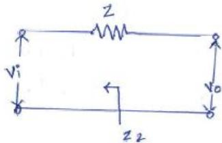
\* Miller's theorem states that, the effect of resistance  $Z$  on the output circuit is the ratio of output voltage  $V_o$  to the current  $I$  which flows from the output to the input.
