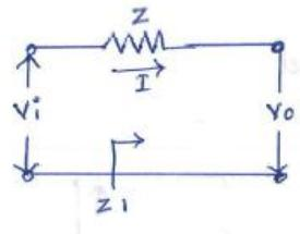
\* Miller's theorem states that, the effect of resistance  $Z$  on the input circuit is a ratio of input voltage  $V_i$  to the current  $I$  which flows from input to the output.
