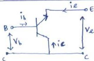
$$(1) \Rightarrow V_b = h_{1c} i_b + h_{rc} V_c \quad \text{--- (7)}$$
