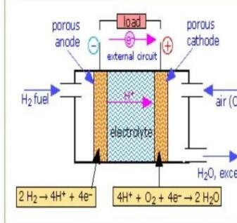
NET REACTION:  $2H_{-} + O_{-} \longrightarrow 2H_{-}O + electrical energy + heat.$
