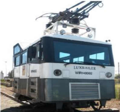
(B) Railway Inspection Vehicle
