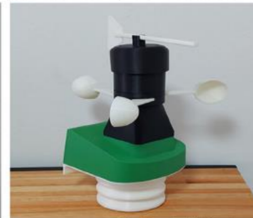
(F) Assembled Weather Station
