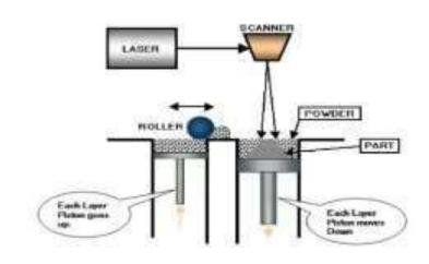
Type: Powder melted with LASER, Requires post processing Material: Nylon, metal
