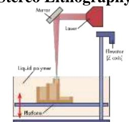
Type: LASER cured resin High resolution, Fragile Material: Resin
