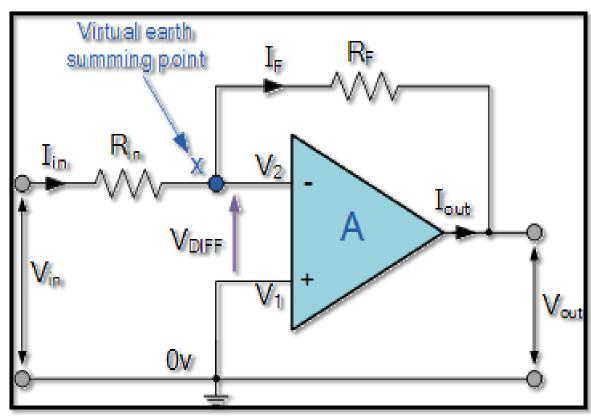
The operational amplifier is connected with feedback to produce a closed loop operation.
