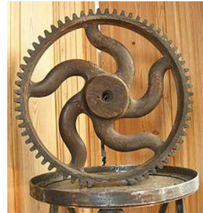
Wooden pattern for a cast-iron gear with curved spokes
