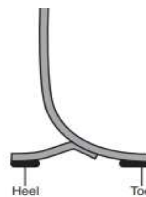
▲ Figure 2-2 ■ The "Flex foot" facilitates gait by its design and composition. The curved blade bends during loading and then assists with propulsion. A change in material affects how much the structure bends and how much energy it provides to subsequent forward movement.
