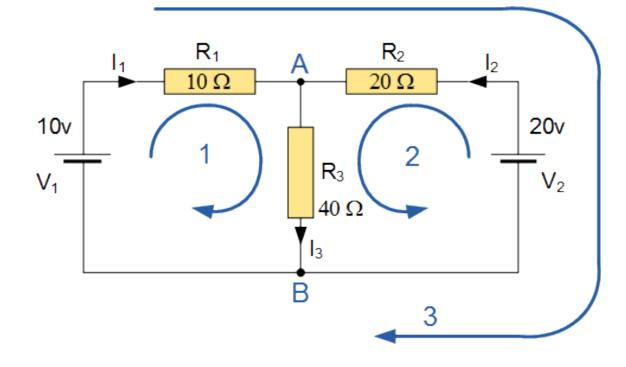
The current flowing in resistor  $R_3$  is given as : -0.143 + 0.429 = 0.286 Amps
