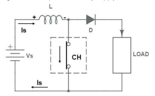
Also, during the TON period, energy is stored in the inductor L. This energy storage in L is essential to boost the load output voltage above the source voltage. Therefore, a large value of L is essential in a step-up chopper.
