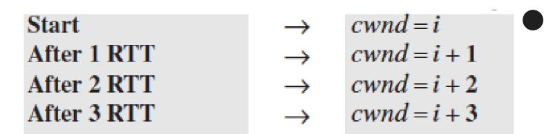
In the congestion-avoidance algorithm, the size of the congestion window increases additively until congestion is detected.
