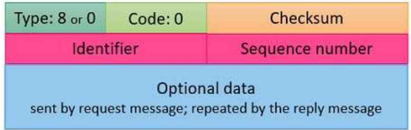
Echo Request and Reply Message Format
