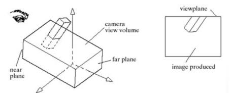
OpenGL provides functions for defining the view volume and its position in the scene, using matrices in the graphics pipeline.
