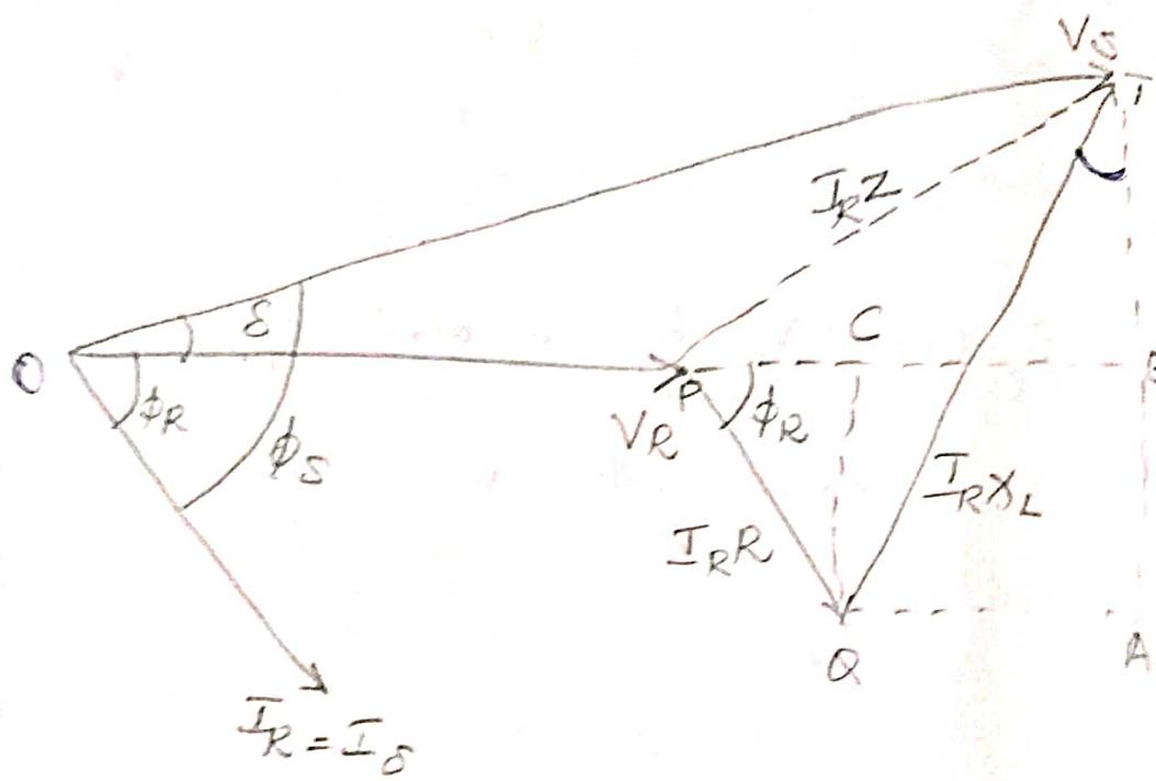
Lagging power factor load is considered to find the tr. efficiency and regulation of the short tr. line.
