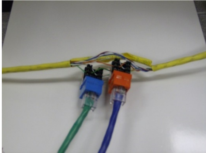
Figure 7.2. Covert Wiretap using Insulation-displacement Connectors
