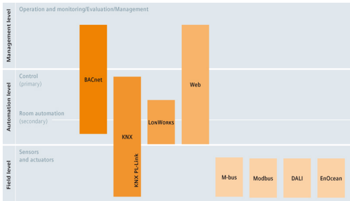
Figure 4.8. BACS Software Architecture (Siemens, 2017)
