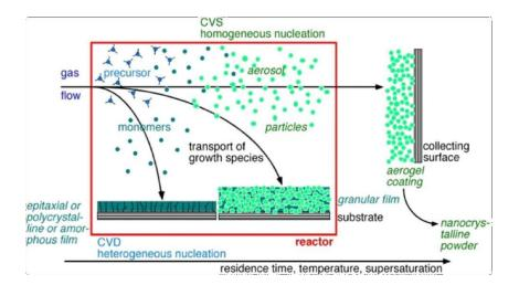
The nanoparticles are extracted from the aerosol by means of filters, thermophoretic collectors, electrostatic precipitators or scrubbing in a liquid. Modifications of the precursor delivery system and the reaction zone allow the synthesis of pure oxides, doped oxides, coated nanoparticles, functionalized nanoparticles and granular films.
