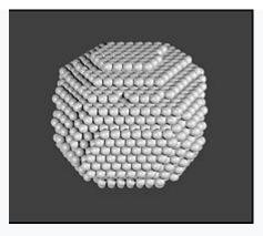
Idealized model of a crystalline nanoparticle of platinum, about 2 nm in diameter, showing individual atoms.
