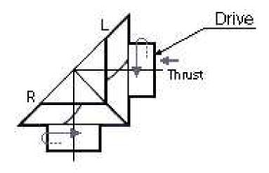
Answer: downward direction, because the thrust act in drive gear pushes the driven gear to downward direction.
