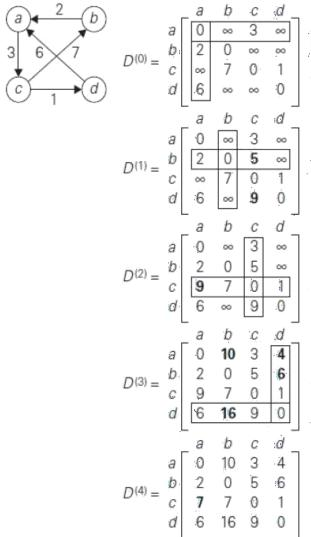
Lengths of the shortest paths with no intermediate vertices ( $D^{(0)}$  is simply the weight matrix).
