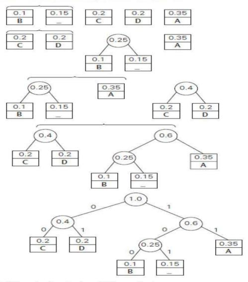
FIGURE 3.18 Example of constructing a Huffman coding tree.
