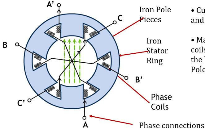
• Current enters coil **A** and leaves coils **A**'
