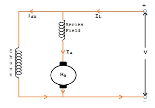
Derive the voltage equation for DC Compound Motor
