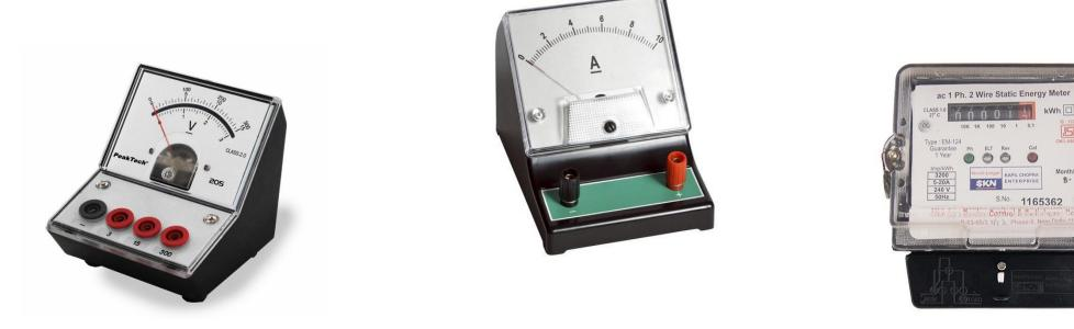
The instruments used for all electrical measurements are called measuring instruments. They include ammeters, voltmeters, wattmeters, energy meters etc.
