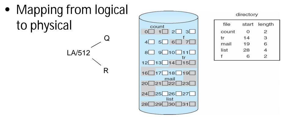
Block to be accessed = Q + starting address Displacement into block = R
