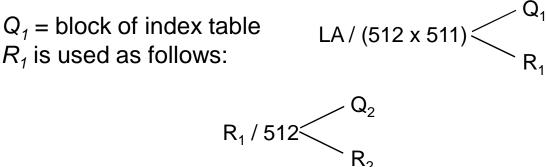
$Q_2$  = displacement into block of index table  $R_2$  displacement into block of file:
