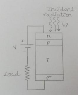
the device is essentially a reverse-biased p-n junction that is operated at voltage close to the breakdown voltage. The photogenerated electrons and holes in the depletion layer, acquire sufficient energy from the field to liberate secondary electrons and holes within the layer by a process q impact - ionization. The secondary electron - hole pair drift in the apposite directions and together with the primary
