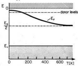
At 0K the Fermi energy is located between the new energy band and  $E_0$ .
