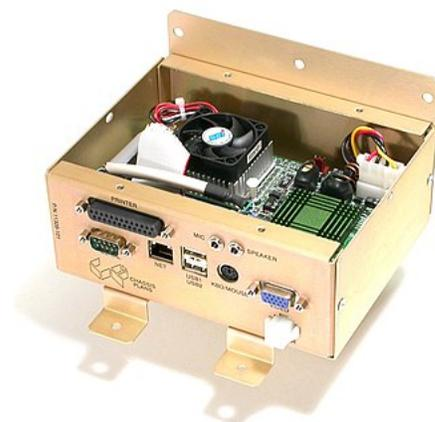
Embedded Computer Sub-Assembly for Accupoll Electronic Voting Machine<sup>[7]</sup>
