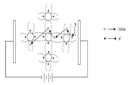
Definition: It is noted that hole current is due to the movement of valence electrons from one covalent bond to another bond.
