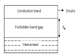
So the valence band is completely filled and the conduction band is empty.
