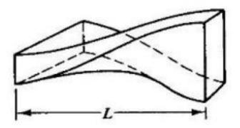
Using waveguide E bends and waveguide H bends and their srap bend counterparts allows the waveguide to be turned through the required angle to meet the mechanical constraints of the overall waveguide system. Waveguide twists are also useful in many applications to ensure the polarisation is correct.
