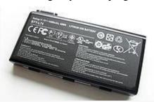
A lithium-ion battery from a laptop computer (176 kJ)
