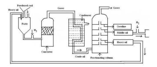
Since the reaction is exothermic the vapours leaving the converter are condensed in the condenser to give synthetic petroleum or crude oil.
