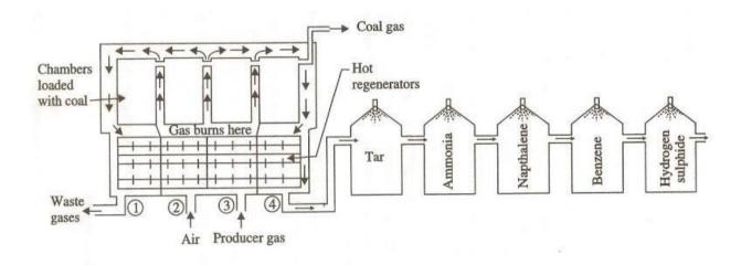
Coal is introduced in to the silica chamber and the chambers are closed. The chambers are heated upto 1200°C by burning pre heated air and the producer gas mixture in the interspaces between the chambers.
