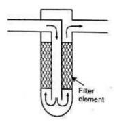
**2. Proportional filters (bypass filters):** In some hydraulic system applications, only a portion of oil is passed through the filter instead of entire volume and the main flow is directly passed without filtration through a restricted passage.
