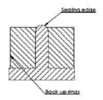
**4.** *Piston cup packings:* Piston cup packings are designed specifically for pistons in reciprocating pumps and pneumatic and hydraulic cylinders. They offer the best service life for this type of application, require a minimum recess space and minimum recess machining, and can be installed easily and quickly.
