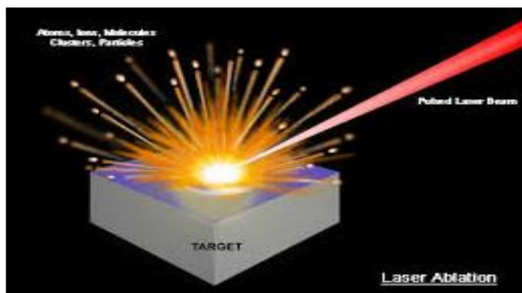
LASiS is a “green” technique for the synthesis of stable NMNp in water or in organic solvents, which does not need stabilizing molecules or other chemicals. So obtained NMNp are highly available for further functionalization or can be used wherever unprotected metal nanoparticles are desired.
