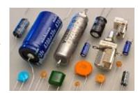
areas of the plates, and is inversely proportional to the separation between the plates. Capacitance also depends on the dielectric constant of the substance separating the plates.
